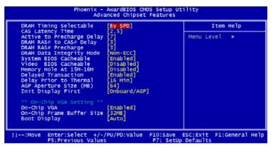
Figure 3.4: Advanced chipset features screen
